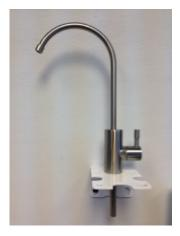
Select a position for the tap on the counter or sink shoulder. The faucet should be located in a position that gives a flow of water into the sink bowl. Ensure (check) that you have enough room below the desired position to connect the tubing (15) to the tap. Using a centre pop (or nail) mark where the centre of the tap stud will be and drill a 12mm hole through the surface. Secure the tap in place by using the fixing kit provided.
