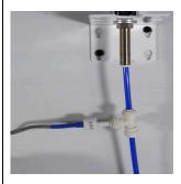
The RHOMBUS system is supplied with an in-line TDS monitor, which allows the operator to monitor the quality of two separate water lines (i.e. the feed and the product. Please follow the instructions that are supplied with the meter. The tee pieces are 'spliced' into the target tubing in the same way that the tubing is fitted on the rest of the system.
