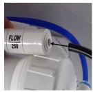
Connect a length of black tubing between the drain clamp (13) and the drain restrictor on the module (this is the white fitting marked 250ml). Remove the horse shoe collet clip and dust cap before trying to push the tubing into the fitting. The ends of the tubing should be cut square with no scratches or burrs.
